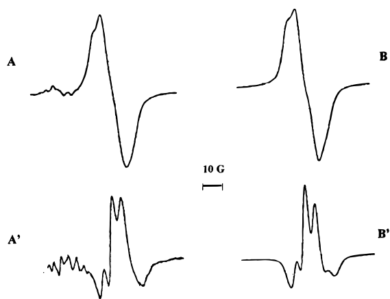
Figure 3. Comparison of the experimental and simulated ESR spectra of the \text{Cp}^*\text{Ti}(\text{}^{13}\text{CH}_3)_3/\text{Ph}_3\text{CB}(\text{C}_6\text{F}_5)_4/\text{Al}(\text{}^{13}\text{CH}_3)_3 system (chlorobenzene, 240 K, [\text{Ti}] = 0.01\text{M} ; B/Ti molar ratio = 1; Al/Ti molar ratio = 3). (A and A') First and second derivative experimental spectra, respectively. (B and B') First and second derivative computer-simulated spectra obtained with a(^{13}\text{C}) = 4.7\text{ G} , respectively.
